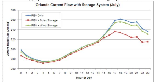
(b) System Current Flow with Storage System
