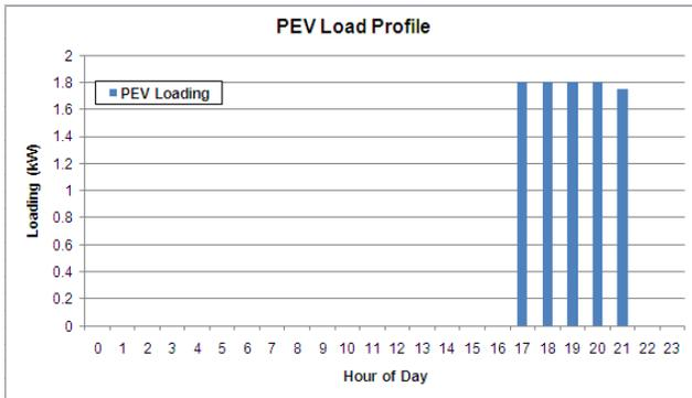
Fig. 2. Typical 120V/15A Charging Profile for PEV
