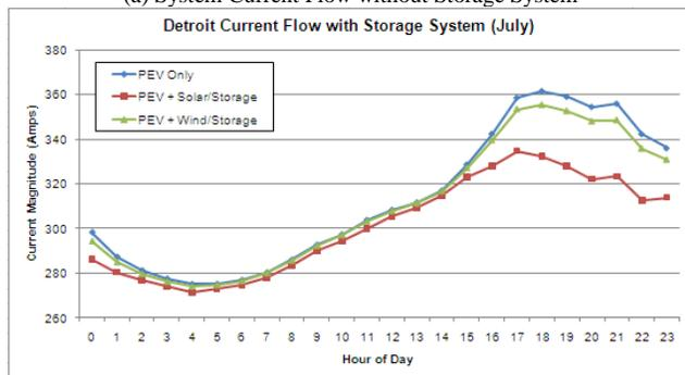
(b) System Current Flow with Storage System
