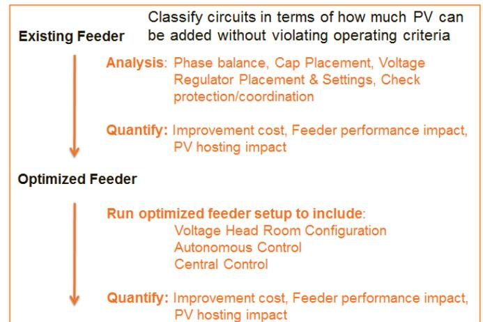
Figure 1. PV Hosting Capacity Automated Analysis
