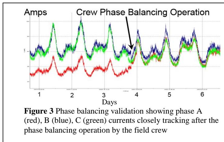
**Figure 3** Phase balancing validation showing phase A (red), B (blue), C (green) currents closely tracking after the phase balancing operation by the field crew
