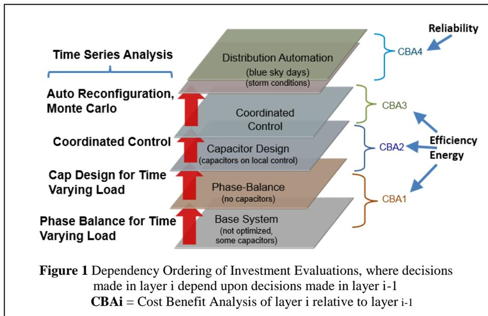
The first two investments, Phase Balance and Cap Design, are made without making large investments in typical smart grid equipment. The **ISM**, with all of the measurement data included, allows ORU to
